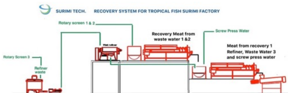
Figure 2.5 Waste recovery system for tropical fish surimi factory
